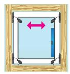
3. Remove the Pumpbag from the top edge and place it together with a second Pumpbag on each side of the frame, on the lower edge. Now adjust the frame vertically by adjusting the pressure in Pumpbag, check with a spirit level.
