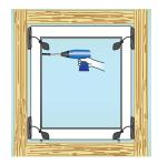
4. Fit the frame with a suitable frame attachment, e.g. Programa frame screw or Indu-Prog frame sleeve.
