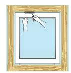
1. Place the window- or the door frame in the opening. The frame must stand on a firm, horizontal surface, use e.g. ESSVE Level screw. Place a Pumpbag on the upper side of the frame to keep the frame in place.
