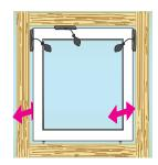
2. Adjust the frame to the correct position. Now place a Pumpbag on each side of the frame, at the top.
