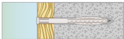
1. Montering i betong
