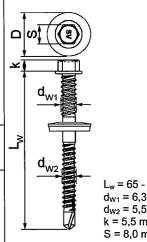
$L_w = 65 - 275 \text{ mm}$  $d_{W1} = 6,3 \text{ mm}$  $d_{W2} = 5.5 \text{ mm}$  $k = 5,5 \, mm$ S = 8,0 mm D = 19,0 mm
