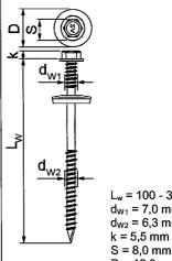
$L_w = 100 - 310 \text{ mm}$  $d_{W1} = 7.0 \text{ mm}$  $d_{W2} = 6.3 \text{ mm}$ S = 8.0 mm $D = 19,0 \, mm$
