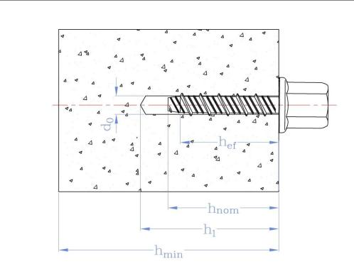
**Drawing A2.** Installed condition for anchors EUS - SSD, EUS - SSI, EUS - SSF, EUS - SSO, EUS - SSU, EUS - SSG, EUS - SSQ, EUS - SSV and EUS - SSG2.
