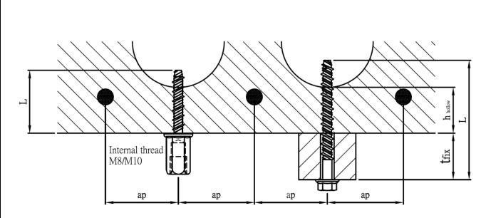
Drawing A4. Installed condition in prestressed hollow core concrete slabs
