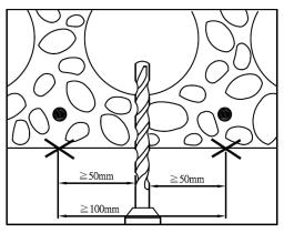
Drawing B4. Installation process in prestressed hollow core concrete slabs
