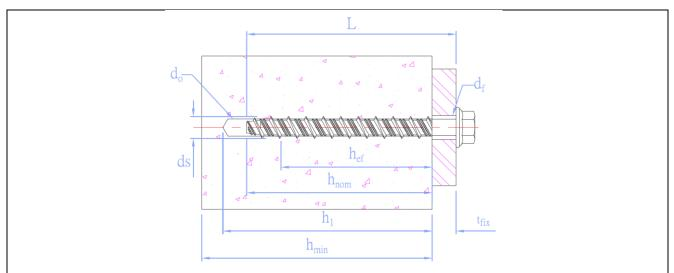
**Drawing B1.** Installed condition for anchors EUS - SSW, EUS - SSR, EUS - SSP, EUS - SSK, EUS - SSH, EUS - SSX, EUS - SST, EUS - SSN and EUS - SSC.
