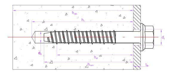
**Drawing A1**. Installed condition in normal weight concrete for anchors EUS - SSW, EUS - SSR, EUS - SSP, EUS - SSK, EUS - SSH, EUS - SSX, EUS - SST, EUS - SSN and EUS - SSC.
