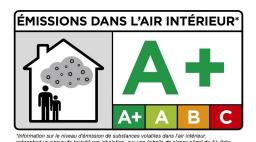
The product was assigned a VOC emission class without taking into account the measurement uncertainty associated with the result. As specified in French Decree no. 2011-321 of March 23, 2011, correct assignment of the VOC emission class is the sole responsibility of the party responsible for distribution of the product in the French market.
